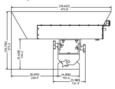
Figure 8. IIT Camera Housing front view
